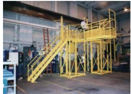
Rail Maintenance: Tip-Down Platform for locomotive maintenance
