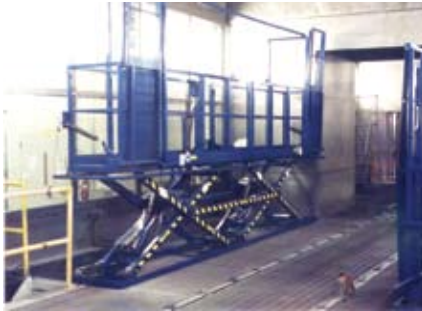
Paint Booth: Scissor Lift with Tip-Down Extension Platforms for Semi Truck Manufacturer
