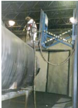
Sand Blast Booth: 3-Axis Lift Designed for blast booths using sand or steel grit
